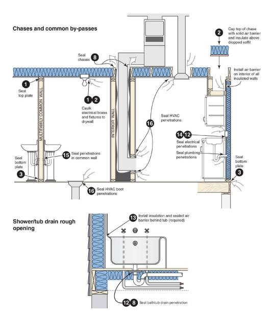
This document is intended solely to help graphically demonstrate the air leakage provisions of section 402.4 of the 2012 IECC. It does not cover all air sealing location or techniques. Other code provisions may be applicable as well.
