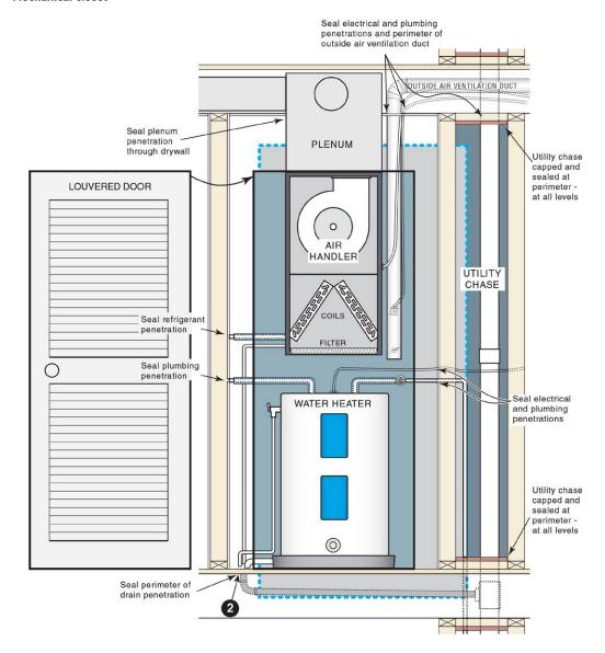
This document is intended solely to help graphically demonstrate the air leakage provisions of section 402.4 of the 2012 IECC. It does not cover all air sealing location or techniques. Other code provisions may be applicable as well.
