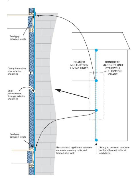
This document is intended solely to help graphically demonstrate the air leakage provisions of section 402.4 of the 2012 IECC. It does not cover all air sealing location or techniques. Other code provisions may be applicable as well.
