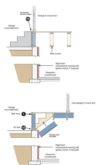
This document is intended solely to help graphically demonstrate the air leakage provisions of section 402.4 of the 2012 IECC. It does not cover all air sealing location or techniques. Other code provisions may be applicable as well.
