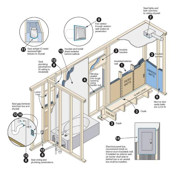
This document is intended solely to help graphically demonstrate the air leakage provisions of section 402.4 of the 2012 IECC. It does not cover all air sealing location or techniques. Other code provisions may be applicable as well.
