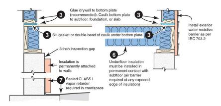
This document is intended solely to help graphically demonstrate the air leakage provisions of section 402.4 of the 2012 IECC. It does not cover all air sealing location or techniques. Other code provisions may be applicable as well.
